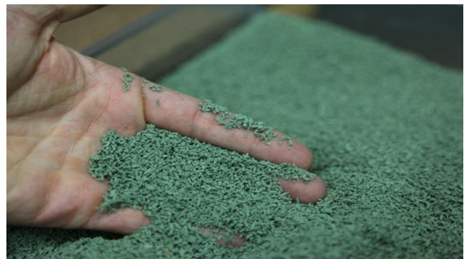
Photo 12: EPDM 'Bionic' infill (Source MELOS)
